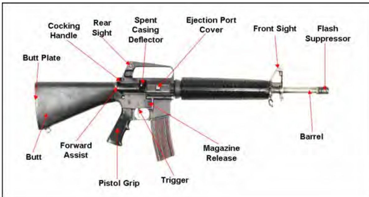
Figure 1 Right Side of the C7 Rifle
